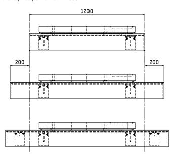
If the stone console is placed on the left or right, an additional console support is required from a width > 1400 mm.
